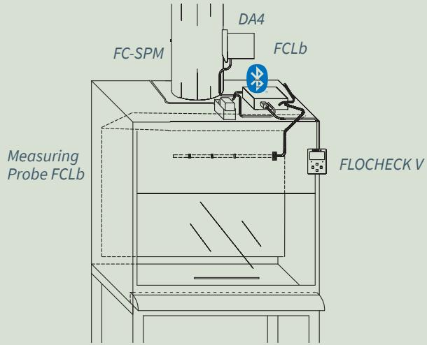
*FCLb with additional equipment for a fume hood. FCLb is equipped with Bluetooth® for access via the LINDINSIDE mobile application.*
